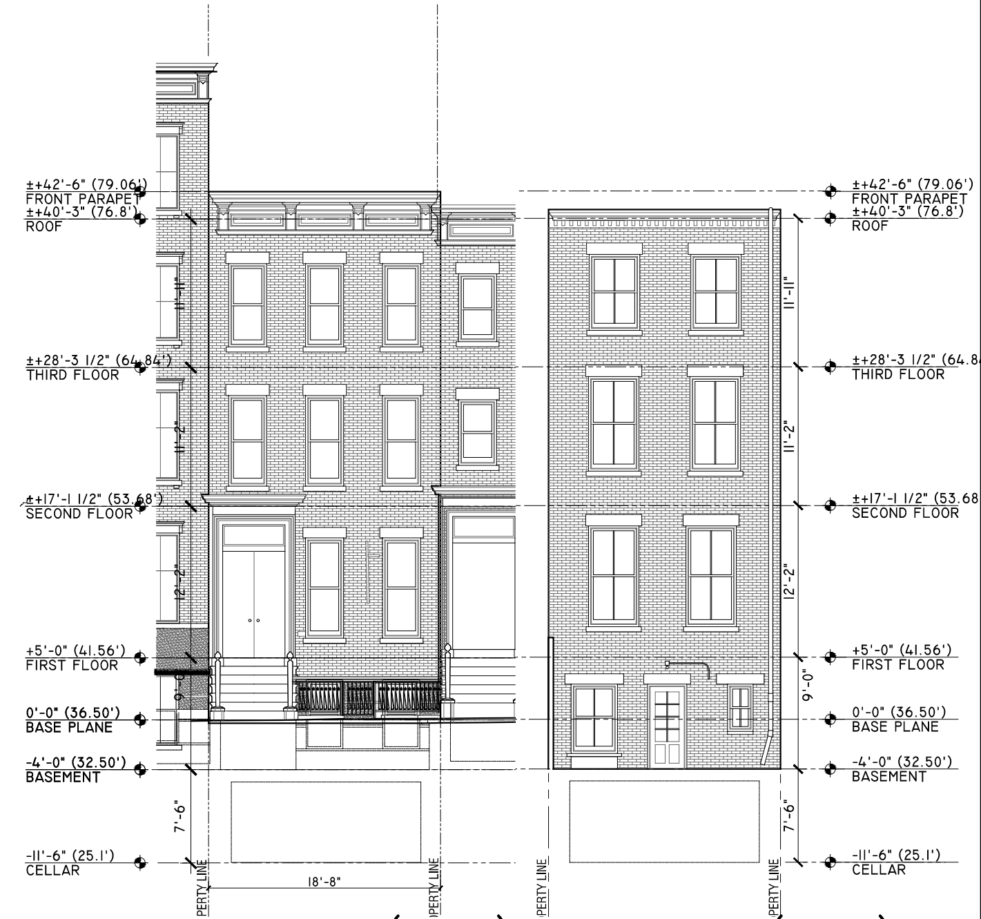
FRONT ELEVATION (NORTH) REAR ELEVATION (SOUTH)
